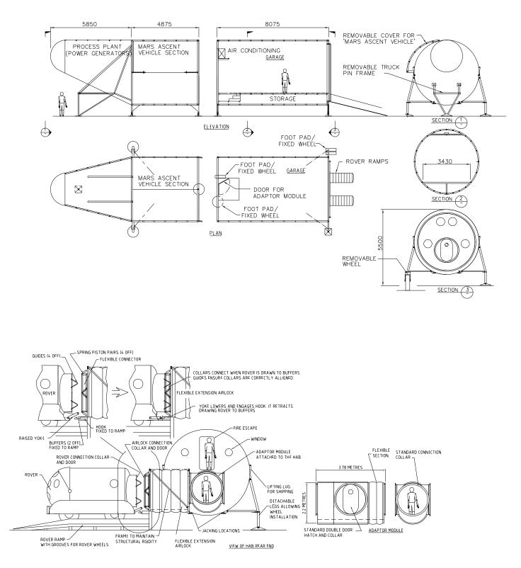
View of Hab rear, adaptor module and flexible extension airlock and rover docking system.
