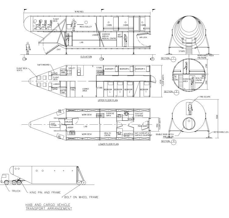
Transportation mode of MARS-OZ modules, using detachable wheels and a prime mover. Two such prime movers will be required to set up the base on the chosen site.
