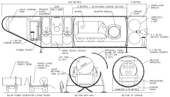
The Cargo Vehicle with a 3 tonne rover and a 3.9 tonne (dry mass) Mars Ascent Vehicle.
