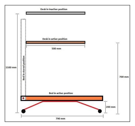
Figure 10: Dimensions of the Combined Bed/Desk System
