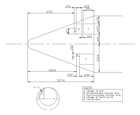
Figure 30: Water system component locations
