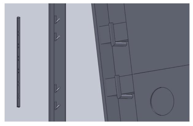
Figure 6: Rails with Close-up Views of Hooks
