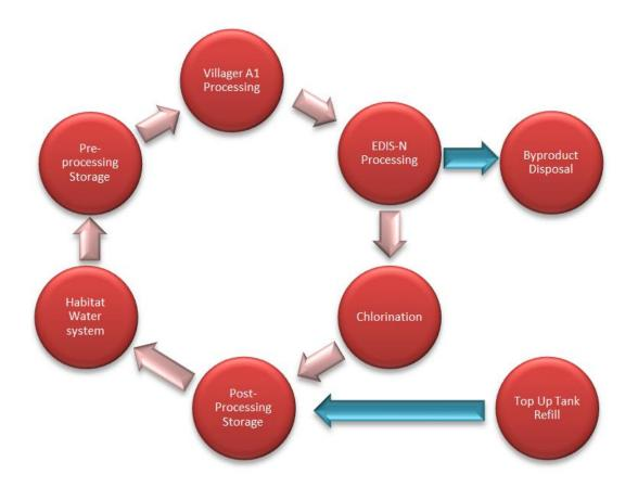
Figure 32: Water Reprocessing Overall System Operations
