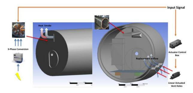
Figure 22: Ventilation and Smoke Evacuation Concept
