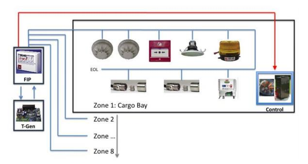
Figure 23: Fire Alarm System using 'Conventional Architecture'
