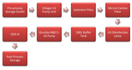
Figure 33: Active Processing Operations
