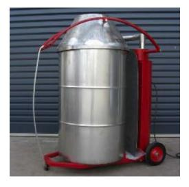
Figure 24: Cyclo Burn Portable Incineration Unit
