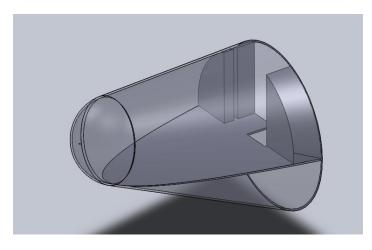
Figure 27: Alternative spacially efficient tank design
