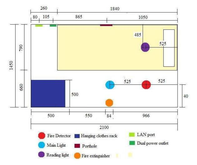
Figure 17: Fully dimensioned bedroom layout for bedrooms 1, 2 and 3. The curved outer wall is located at the top of the figure and the door to the cabin is located at the bottom of the figure. All measurements are in millimetres (mm).
