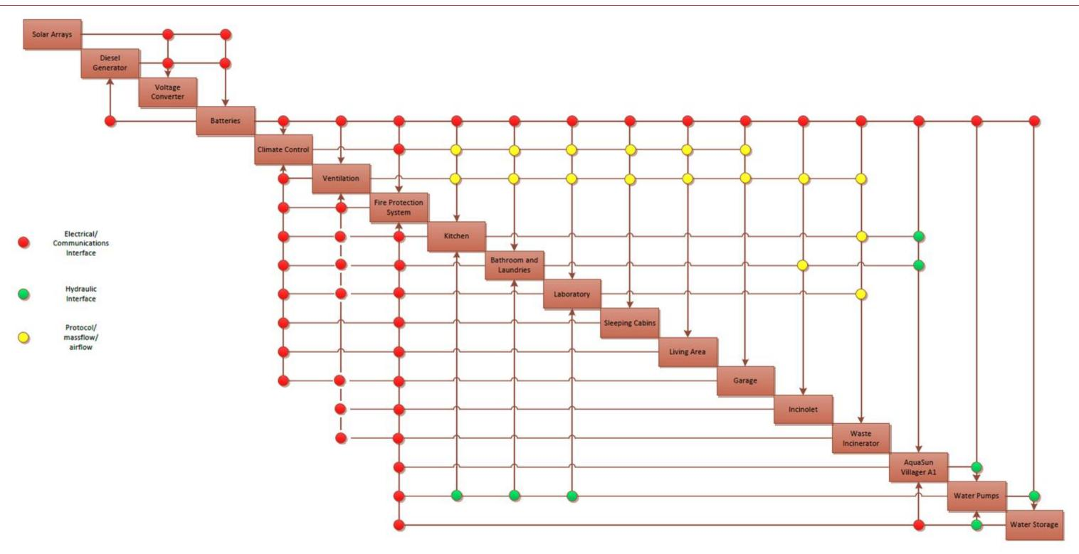
Figure 40: N-squared chart demonstrating design integration and processes
