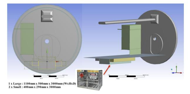
Figure 21: In-floor Storage Space and Compartments
