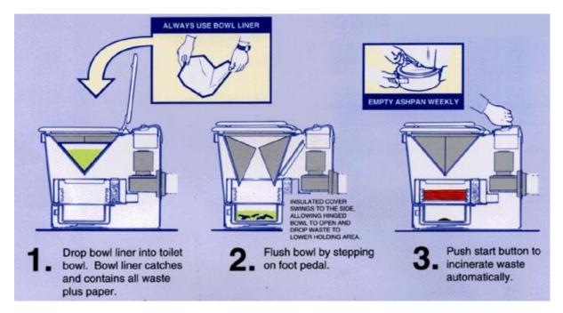
Figure 25: Diagram for using the INCINOLET toilet (Source: http://incinolet.com)
