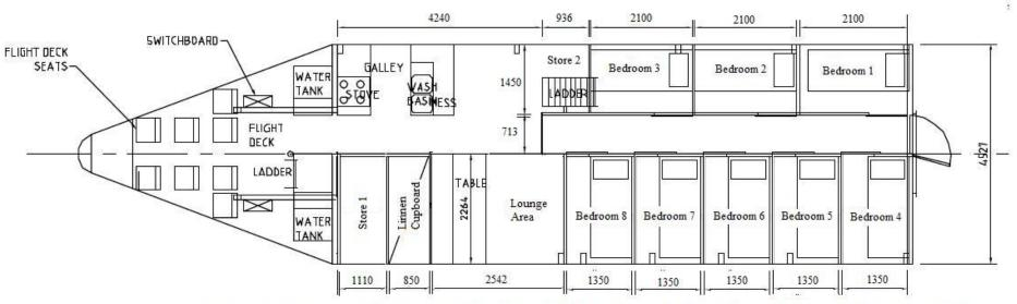
Each cabin wall, the cabin doors and the corridor walls are indicated in the measurements by dounble dashes. The thickness of each of these is 50mm
