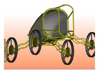
Figure 2: Rear view showing space frame for work area. This may be expanded with an inflatable structure.
