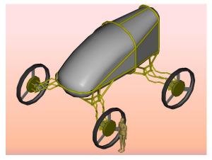
Figure 1: The Wombat Preliminary Design. 6' Human for scale. Note wide wheelbase and large rims.
