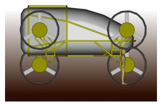
Figure 5: Split view, wheels deployed/folded
