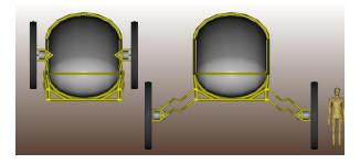
Figure 3: Front view of wheels deployed/stowed.
