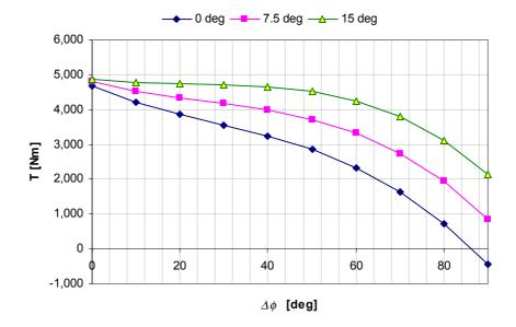
Static Torque requirment on each wheel versus obstacle traverse angle for  $r_{\theta}$  = 250 mm for varying slope angle  $\theta$
