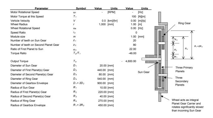
Figure 3 First order design calculation for a planetary (epicylical) gear train. More detailed calculations accounting for tooth fatigue and pitting and more evenly distributing loads will be needed to finalise module selection and gear sizes.
