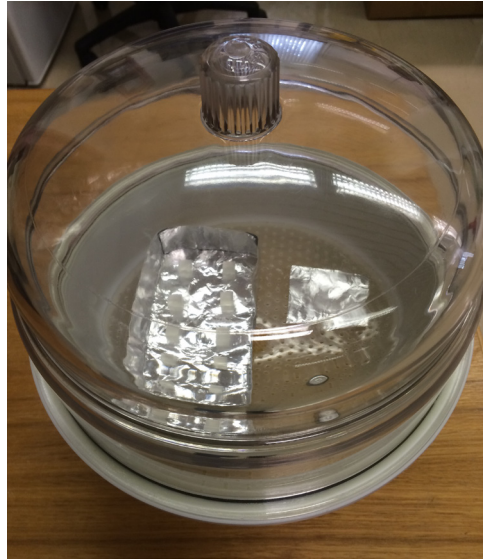
Fig. 6: Outgassing samples and aluminium foil stored in desiccator when not in vacuum chamber.
