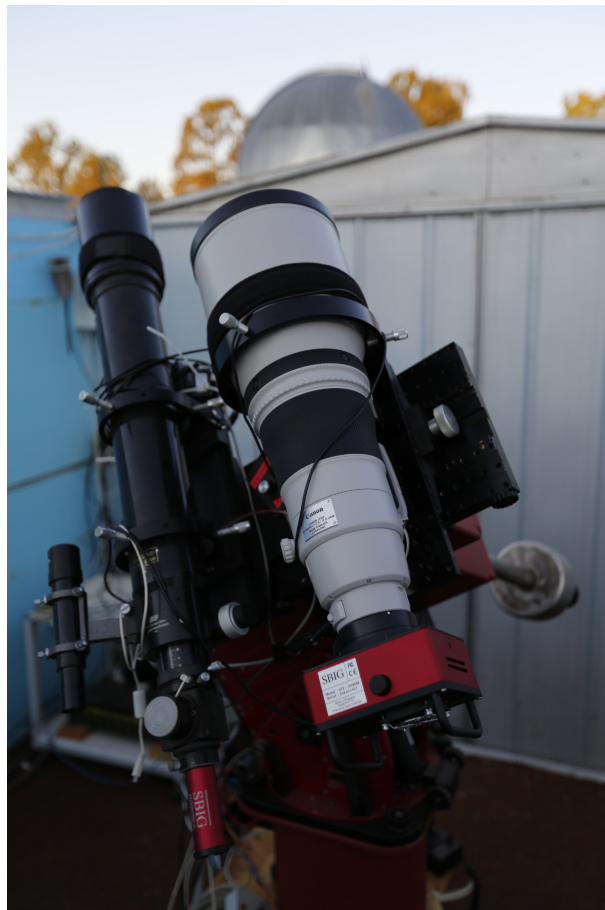
Fig. 1: The Huntsman Eye, a prototype imaging unit of the Huntsman Telephoto Array, during on-sky testing in September 2014
