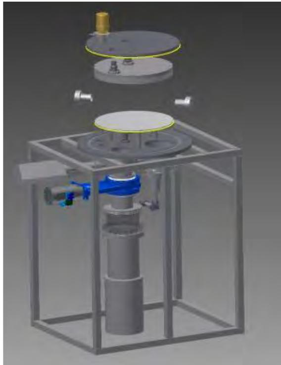
*Figure 2: Assembly CAD rendering, exploded view of the small vacuum chamber*
