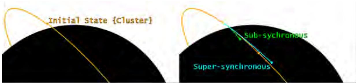
Fig. 5: Visualisation of the first impulsive manoeuvre and satellites phase from the initial state
