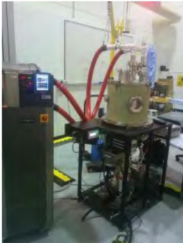
Figure 4: Thermal Vacuum Chamber Lab at UNSW Canberra
