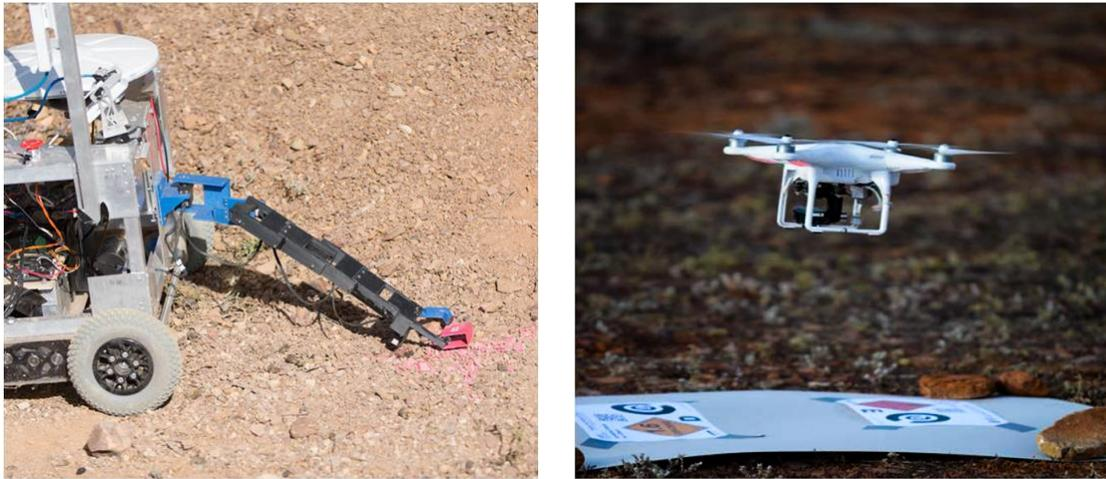
Figure 5: UNSW Rover collecting target object during Sample Return task (left). Phantom 2 quadrotor above horizontal visual targets (right).
