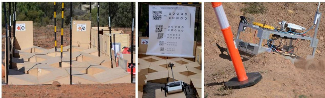
Figure 3: (Left to right) Continuous 15° pitch/roll ramps. Mascot at the far-field acuity test. UNSW Rover traversing irregular terrain.
