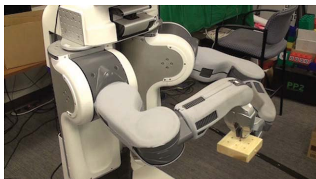
Figure 17. The PR2 executing the peg-insertion learning-assessment benchmark.
