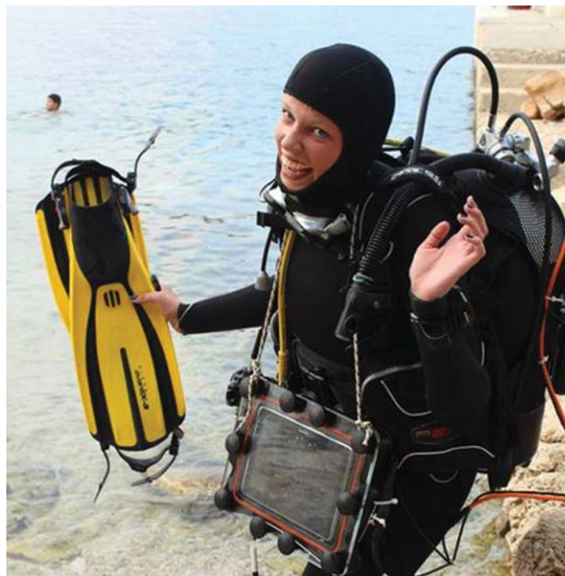
Figure 4. A diver with the underwater tablet preparing to start the experiments. The underwater casing, rated for depths up to 50 m, allows touchscreen functionality when using tablets with inductive screens. The tablet is linked to the surface via the acoustic modem mounted on the diving tank.
