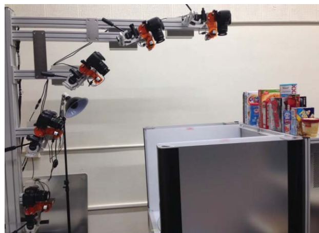
Figure 9. The BigBIRD object-scanning rig: the box contains a computer-controlled turntable.
