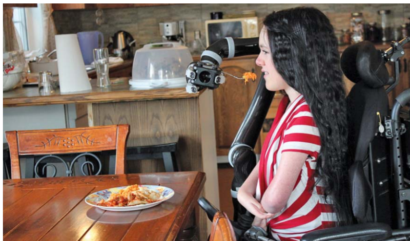
Figure 1. The JACO arm can provide those with upper-body disabilities more independence, enabling them to perform everyday tasks, such as eating, on their own.
