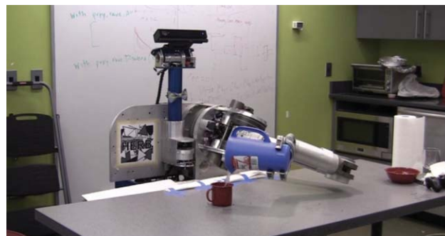
Figure 12. The HERB robot implementing the pitcher–mug benchmark.
