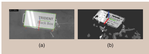
Figure 4. (a) The camera image with manually initialized corners and estimated box pose. (b) Ground truth box pose with the point cloud obtained with the stereo camera.
