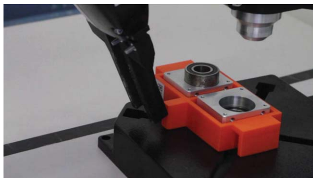
Figure 3. A robot assembling an aid tray for force fitting (TBM1@Work). The picture comes from the RoCKIn consortium.
