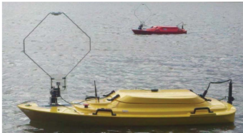
Figure 8. Researchers at the Robotic Sensor Network Laboratory at the University of Minnesota have built a network of autonomous surface vehicles that can collaboratively find and track radio-tagged invasive fish. The tracking algorithm presented by [4] can break and reestablish communication while achieving desired levels of tracking performance. (Photo courtesy of RSN Lab, University of Minnesota.)
