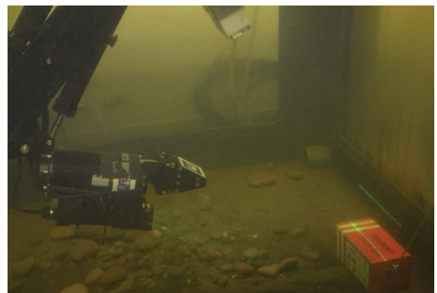
Figure 3. The physical benchmarking system: a water tank, a Lightweight ARM5E manipulator, a stereo camera, a laser stripe projector, and black box mockup.
