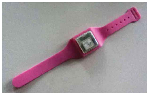
Figure 4. The wearable sensing device used for the WHARF data set recordings. The device, equipped with a triaxial accelerometer, is worn on the right wrist.
