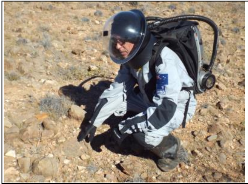
Fig. 5: The high flexibility of the VSSEC suits enables the wearing to easily crouch down while inspecting rocks on the ground.
