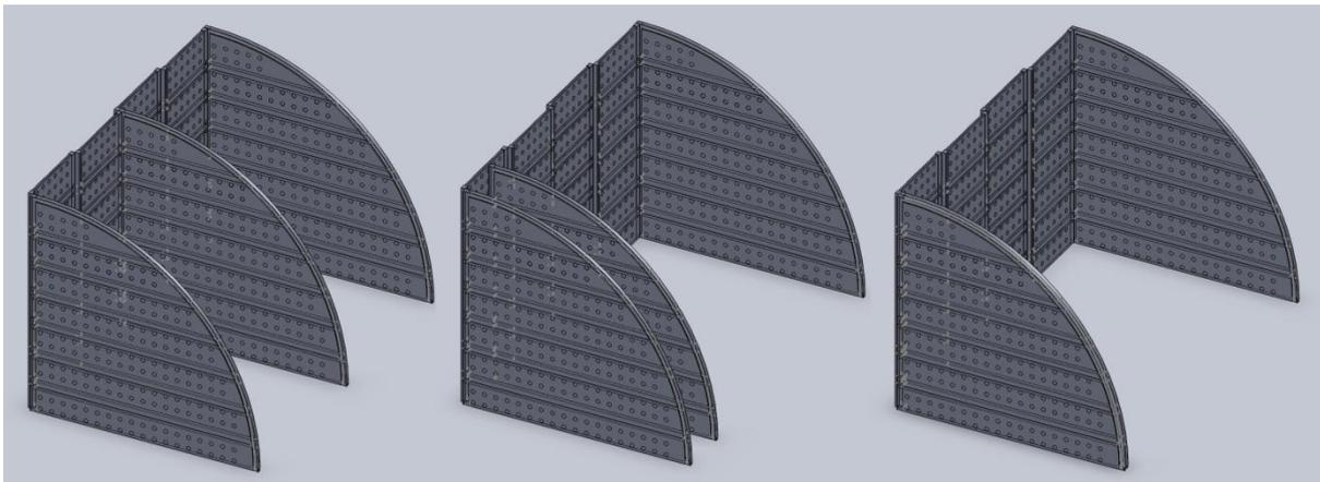
*Figure 15: Conversion from two single rooms to a double room*
