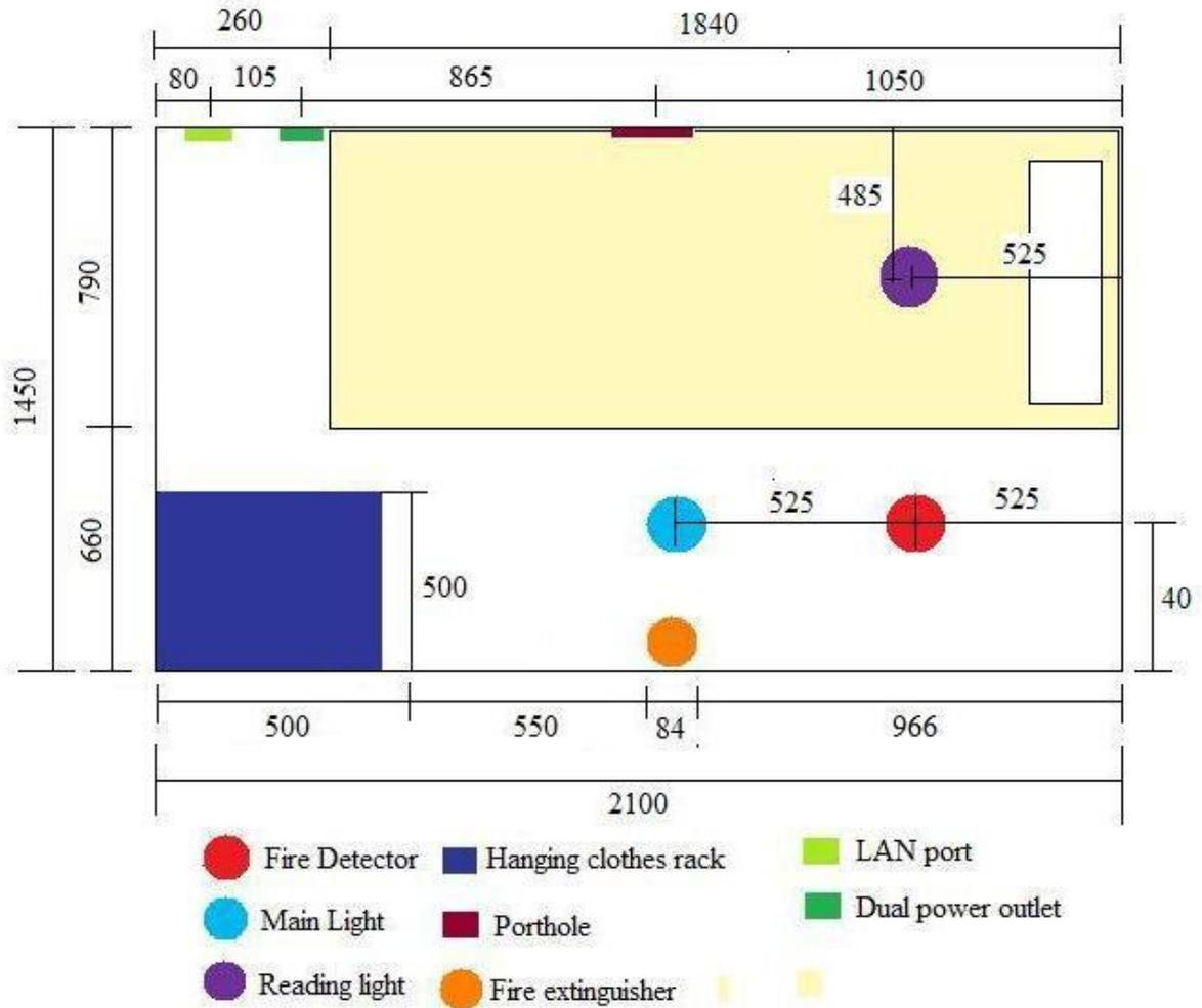
Figure 17: Fully dimensioned bedroom layout for bedrooms 1, 2 and 3. The curved outer wall is located at the top of the figure and the door to the cabin is located at the bottom of the figure. All measurements are in millimetres (mm).
