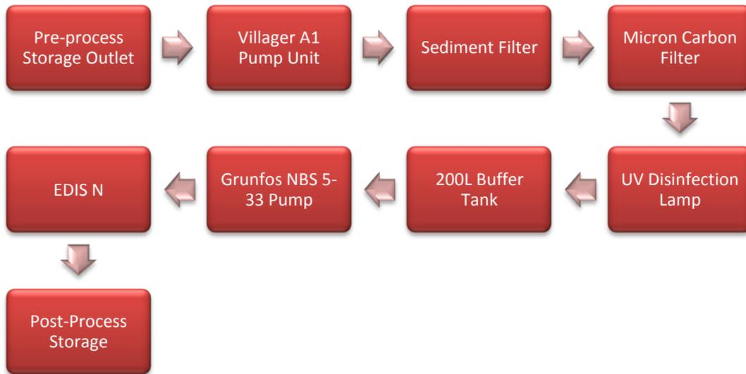
Figure 33: Active Processing Operations
