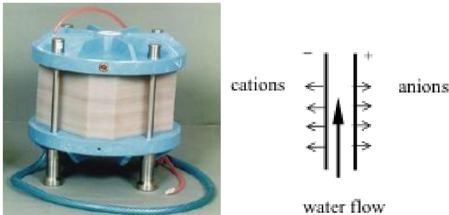
Figure 29: EDIS 'N' (50L/h) EIKOS (Left) and Electrodialysis Process (Pilat 2001)
