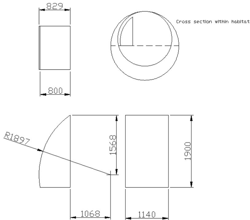
**Figure 26: Port-side water tank schematic showing fitment within habitat frame.**
