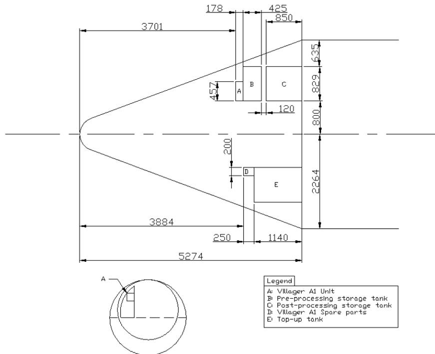
Figure 30: Water system component locations
