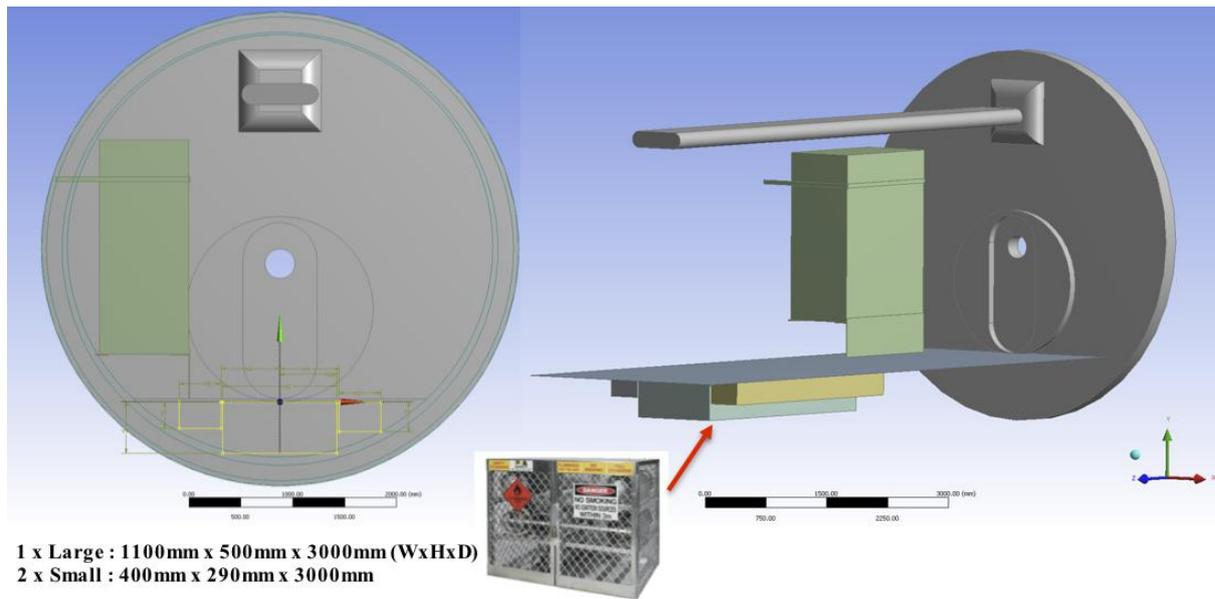
*Figure 21: In-floor Storage Space and Compartments*
