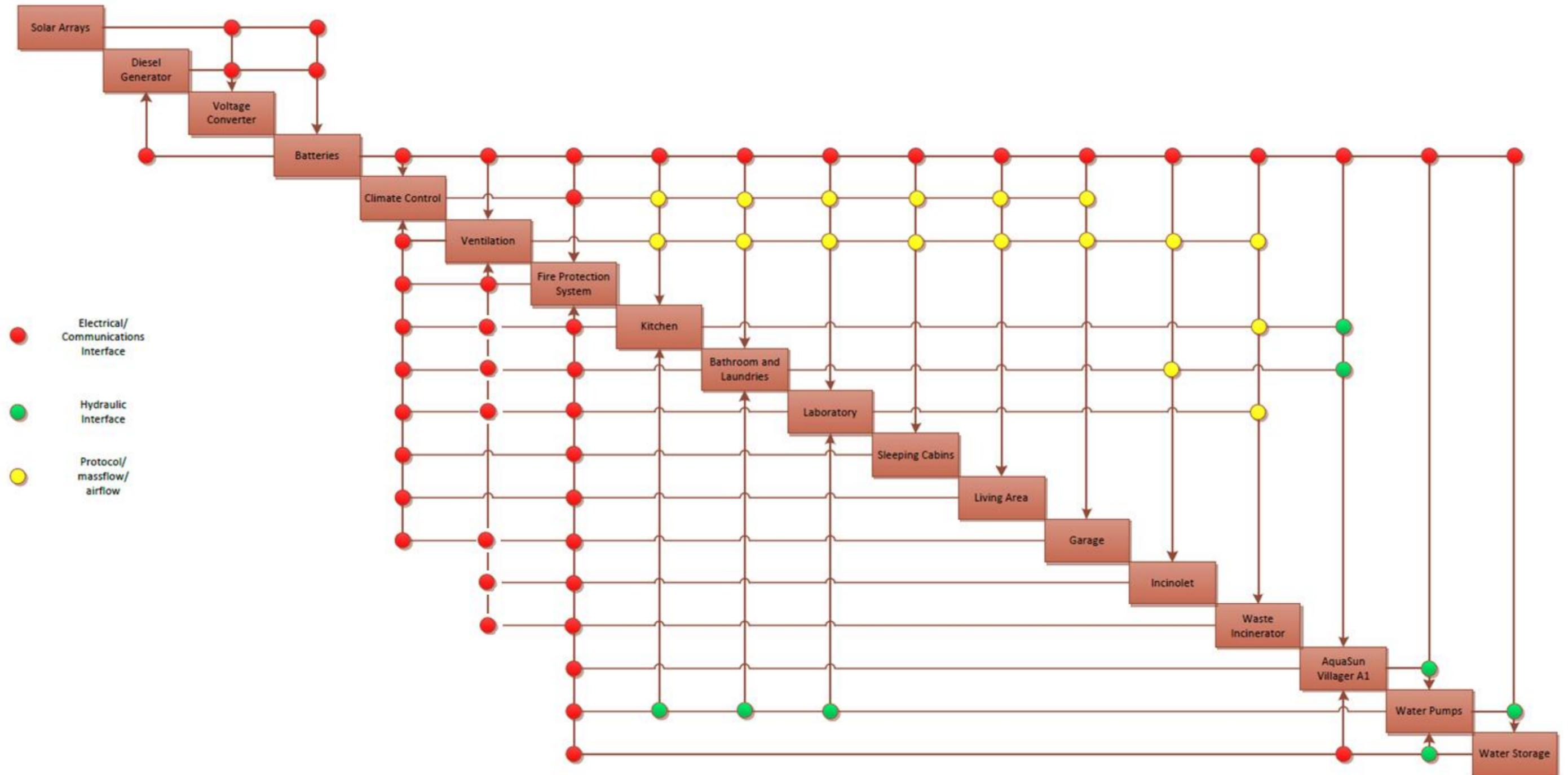
Figure 40: N-squared chart demonstrating design integration and processes
