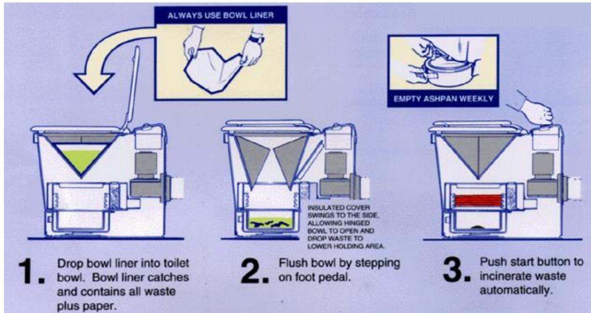
Figure 25: Diagram for using the INCINOLET toilet (Source: <http://incinolet.com>)
