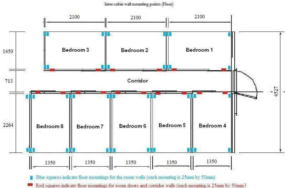
*Figure 16: A plan view of the bedrooms and corridor displaying the mounting points for the inter-cabin walls. NOTE: All measurements are in millimetres (mm).*
