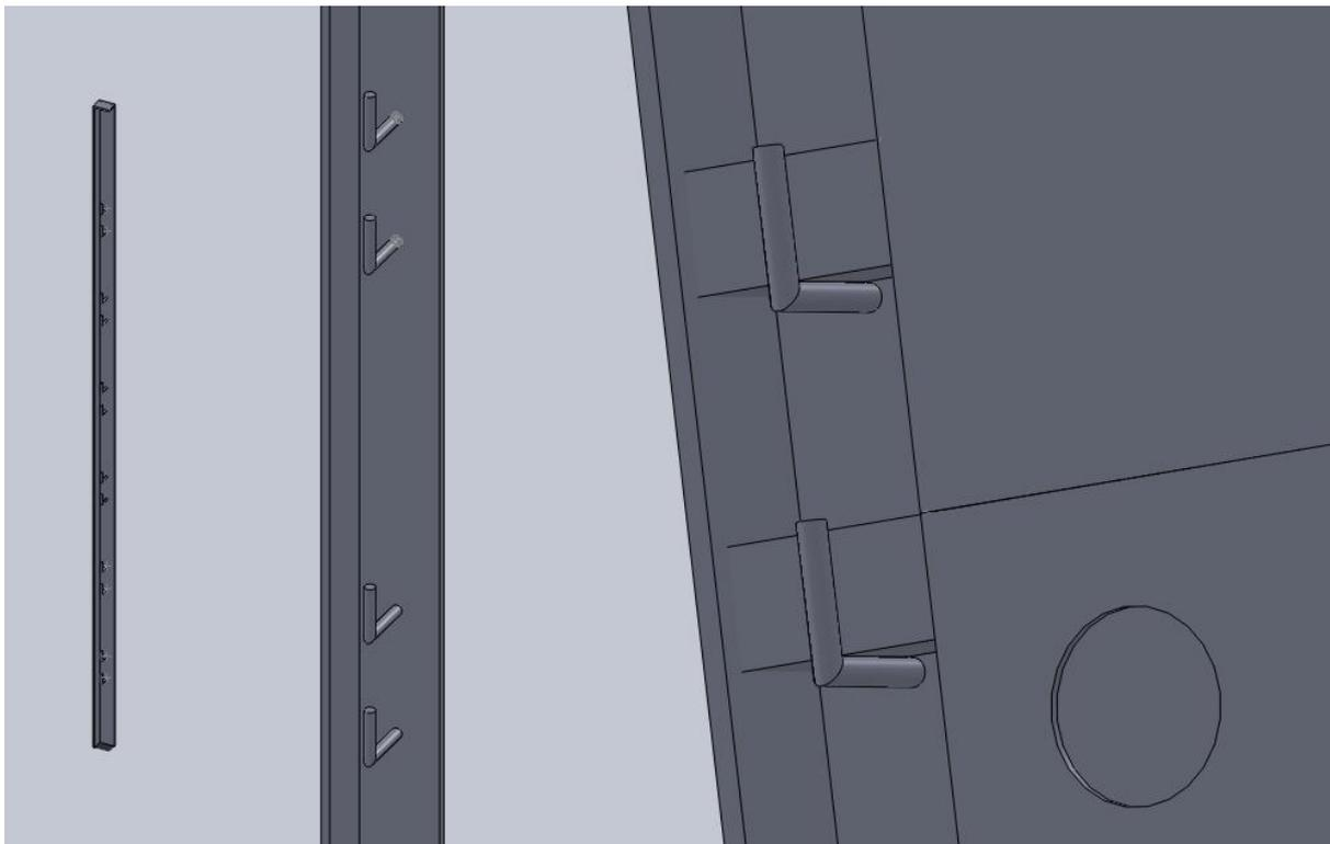
*Figure 6: Rails with Close-up Views of Hooks*
