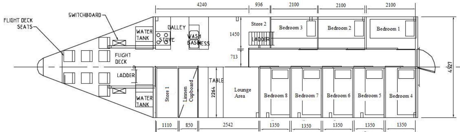
Each cabin wall, the cabin doors and the corridor walls are indicated in the measurements by double dashes. The thickness of each of these is 50mm
