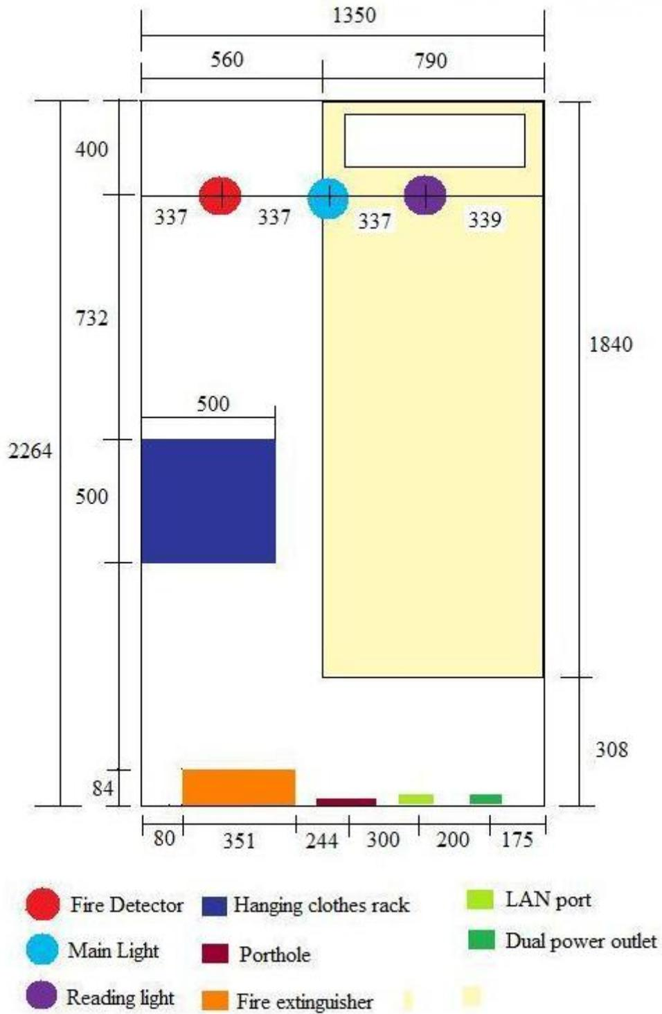
Figure 18: Fully dimensioned bedroom layout for bedrooms 4, 5, 6, 7 and 8. The cabin door is located at the top of the figure and the curved outer wall is located at the bottom of the figure. All measurements are in millimetres (mm).
